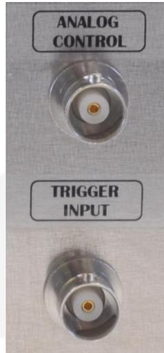
**Figure 7:** Trigger and Analog input connectors
