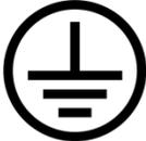
Protective Ground Conductor Terminal
