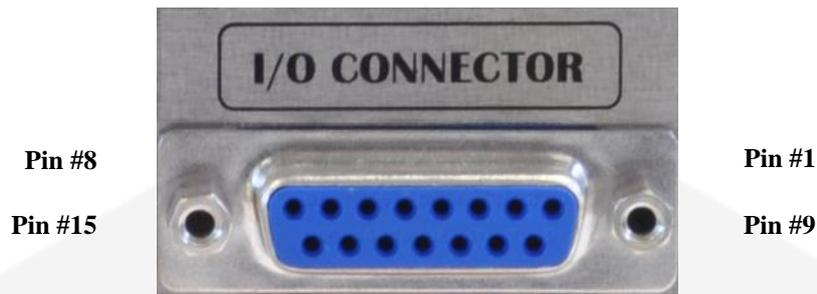
**Figure 3:** I/O Connector
