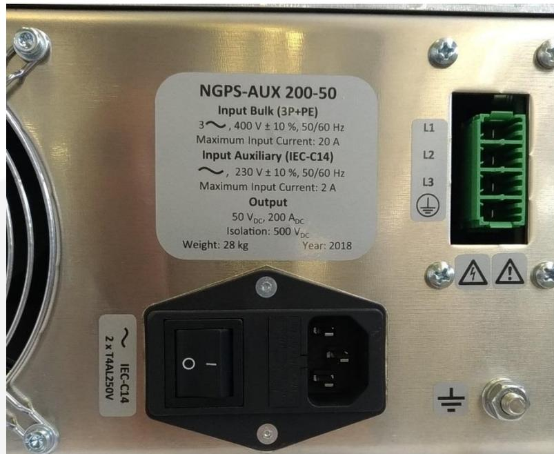
**Figure 12:** NGPS-AUX additional single-phase input
