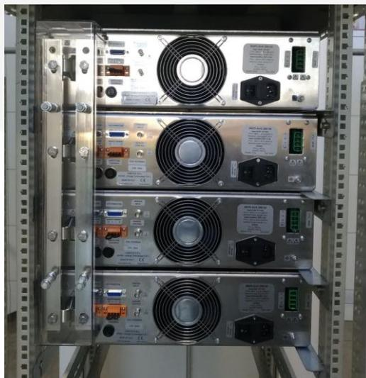
In order to parallel the output terminals, bar connections (as in the pictures above) have to be preferred over cable connections.
