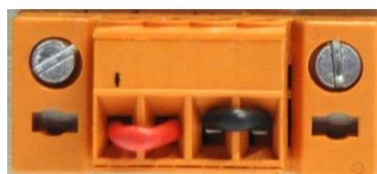
**Figure 5:** Factory mating connector
